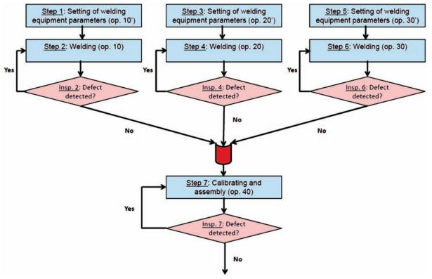
Figure 5 – Integrated the first inspection procedure
