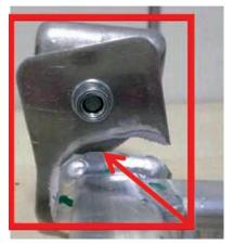
Figure 7 – Damage in a car fender
