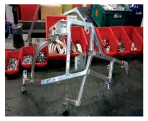
**Figure 3** – Calibrating and assembly operation (operation 40)
