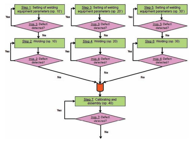
Figure 6 – Integrated the second inspection procedure
