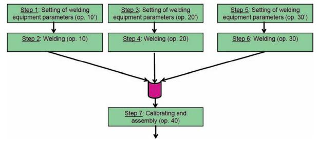
Figure 4 – Flow chart representing the production process
